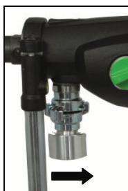
Dust which occurs during your work is hazardous to health. That is why it is advisable to use a deduster and to wear a dust mask on dry drilling. Place the adapter for the dedusting unit onto the tool's connector and turn into the direction of the arrow up to the stop. As a suitable wet/dry deduster, our DSS 25 A is available as add-on. The use of a dedusting system is also a prerequisite for optimal cutting performance of the bit (air cooling).
