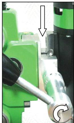
The **ETN 162/3** is equipped with a special accommodation for the diamond drill rig BST 182 V/S. For mounting the tool to the drill rig, the handle may remain at its place.
