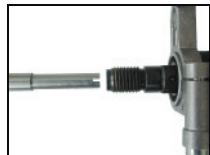
Insert the centering point so that the recesses in the centering point latch on the catches of the working spindle.
