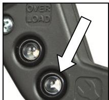
In addition there is a service indicator on the operating handle which indicates in advance that the machine is about to shut down due to worn carbon brushes. After the indicator lights up, you can use the tool for approximately 1 day. Then the carbon brushes should be replaced.
